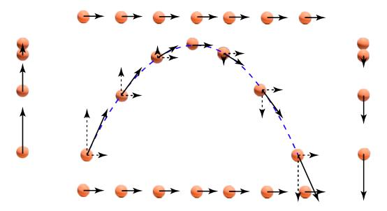
The acceleration of the projectile (in yellow) is always straight down and has a magnitude of 9.81 m/s<sup>2</sup>.
