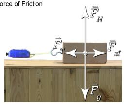
Now I pull until the block moves. The first part is all static friction, when the block is stationary and the force of tension equals the force of static friction. This means the maximum force of static friction is also the force of tension. Then the block starts to move and the friction switches to kinetic. After the block starts to move, the force of tension decreases, because the coefficient of static friction is greater than the coefficient of kinetic
