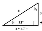
A *Right Triangle* is a triangle with a right angle or 90° angle. This is a right triangle and the symbol for the right angle is shown here.
