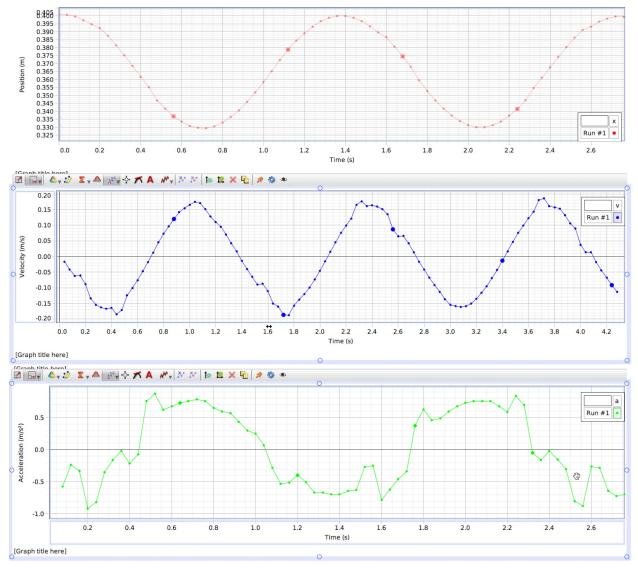
Determining the period using the time for two cycles:  $2T = 2.72 \sec \Rightarrow T = \frac{2.72}{2} = 1.36 \sec t$
