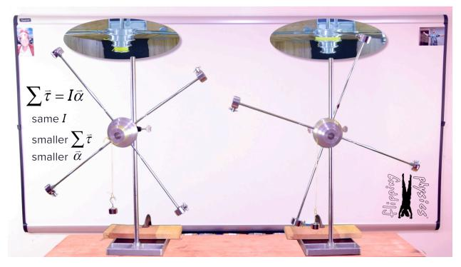
Our last set of demonstrations has both demonstrators with identical rotational inertias and masses hanging from the smallest pulleys. Also, both demonstrators have a 100-gram mass hanging over the left side of the pulley. However, the demonstrator on the right has a second mass, a 200-gram mass, hanging over the right side of the pulley. This means the demonstrator on the right has two different masses hanging off of the smallest pulley.
