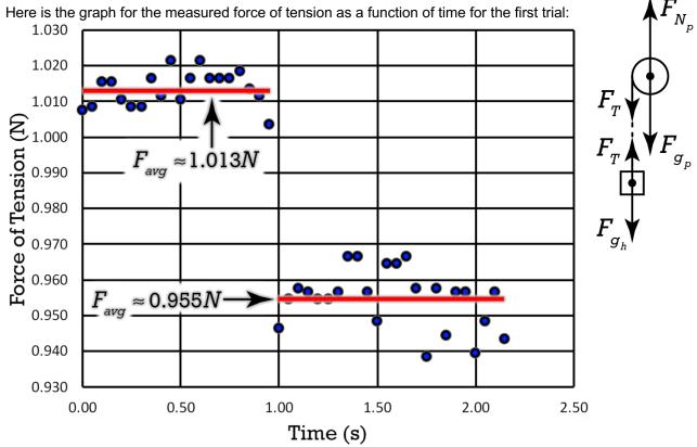
The hanging mass is released just before 1.00 seconds. The acceleration of the system before that is zero because the system is at rest. Therefore:
