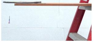
Knowns:  $m_d = 0.0053 kg; v_{di} = 16.5 \frac{m}{s}; m_c = 0.0718 kg; x = 0.287m; L_c = 0.339m; \theta_f = ?$
