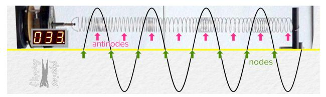
In case you wanted to perform some calculations, the length of the coils of the stretched spring is 41.8 cm.
