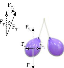
$$\sum F_{y} = F_{T_{y}} - F_{g} = ma_{y} = m(0) = 0 \Rightarrow F_{T_{y}} = F_{g} \Rightarrow F_{T} \cos \theta = mg \Rightarrow F_{T} = \frac{mg}{\cos \theta}$$
