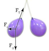
Break Force of Tension into its components.
