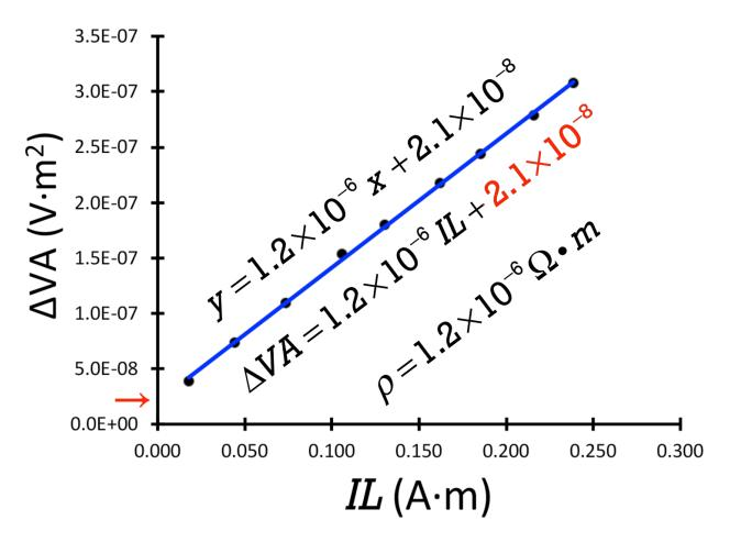
The resistivity we get from our experiment is roughly  $1.2 \times 10^{-6} \Omega \cdot m$ , which is right in the range we expect because the published value for the resistivity for nichrome at 20°C is in the range  $1.0 - 1.5 \times 10^{-6} \Omega \cdot m^{-1}$ .
