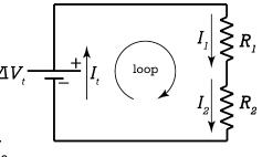
According to Kirchhoff's Loop Rule, a charge moving d with the same electric potential energy it started with, therefore, the electric potential difference all the way around a loop is equal to zero. If we define the loop in a clockwise direction in our circuit, Kirchhoff's Loop Rule looks like this:  $\Delta V_{loop} = \mathbf{0} = \Delta V_t - \Delta V_1 + \Delta V_2 \Rightarrow \Delta V_t = \Delta V_1 + \Delta V$
