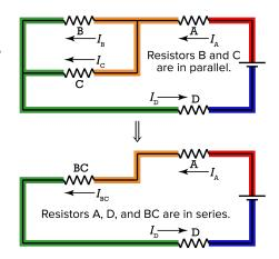
Resistor B is now removed from the circuit, and there is no connection between the wires that were attached to it. The new circuit diagram is shown.
