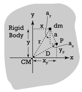
The rotational inertia of the rigid object about its center of mass and about the axis which passes through point P are:
