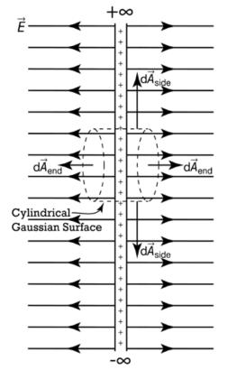
$$\Rightarrow \Phi_{E} = \int_{\text{side}} E dA \cos \theta_{\text{side}} + \int_{\substack{\text{left} \\ \text{end}}} E dA \cos \theta_{\text{end}} + \int_{\substack{\text{right} \\ \text{end}}} E dA \cos \theta_{\text{end}} = \frac{q_{\text{in}}}{\epsilon_{\emptyset}}$$
