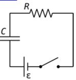
At time initial,  $t_i = 0$ , we close the switch. We are *charging a capacitor through a resistor*.
