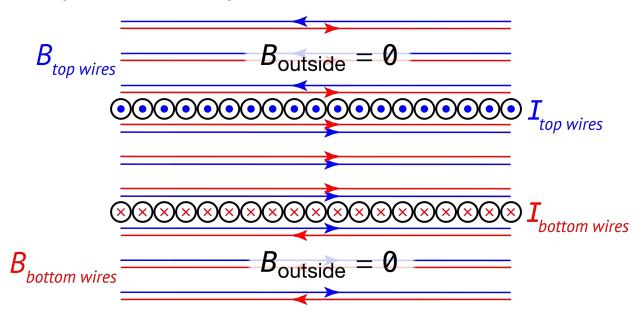
Outside the solenoid, the magnetic field caused by the current in the top wires completely cancels out the magnetic field caused by the bottom wires. In other words, an ideal solenoid has zero magnetic field outside the cylinder of the solenoid. (ideal solenoid below)
