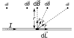
However, now realize that there are, for an infinitely long, straight, current carrying wire, an infinite number of dL's and all of their magnetic fields add up to cause the magnetic field to have a uniform value at a distance r straight out from the wire. And, the magnitude of the magnetic field decreases as r, the distance from the wire, increases.
