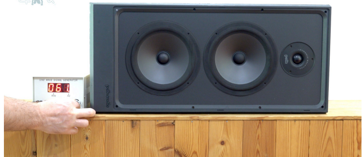
That rattling sound is standing wave patterns at resonance frequencies of the speaker.
