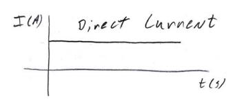
Direct Current, DC: Direction and magnitude of the current is constant. Large power loss over distance.
