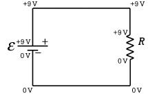
the electric potential difference across the resistor also has a magnitude of 9 volts. In other words, in this circuit with two circuit elements, the two elements, the battery and the resistor, both have the same magnitude electric potential difference.
