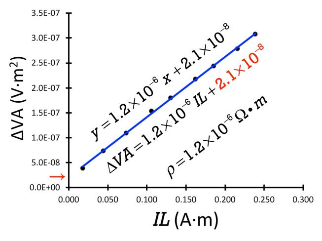
The resistivity we get from our experiment is roughly 1.2 x  $10^{-6} \Omega \cdot m$ , which is right in the range we expect because the published value for the resistivity for nichrome at  $20^{\circ}$ C is in the range  $1.0 - 1.5 \times 10^{-6} \Omega \cdot m$ .
