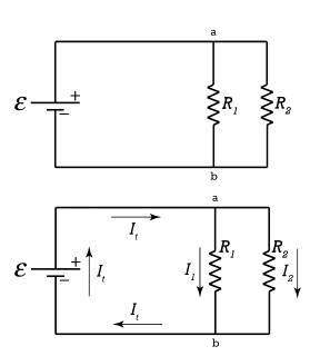
charge in the circuit and see which direction the Law of Charges defines electric force direction on the charge. This means current will go to the right through the top wire, to the left through the bottom wire, and down through both resistors. Let's label those currents as current 1 through resistor 1, current 2 through resistor 2, and current t through the battery because it is the current through the terminals of the battery.
