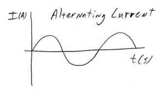
Alternating Current, AC: Direction and magnitude of the current changes. Has a frequency like a sine or cosine wave. Less power loss over distance.
