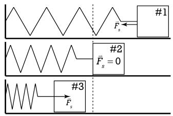
At positions 1 and 3, displacement from equilibrium position, x, will have a maximum magnitude. That means, according to Hooke's Law,  $\vec{F}_s = -k\vec{x}$ , the spring force will also have it's maximum magnitude at positions 1 and 3. If we sum the forces in the x direction,  $\sum F_x = F_s = ma_x$ , we can see the acceleration will also have its maximum magnitude at positions 1 and 3.
