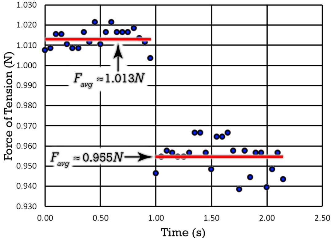
The hanging mass is released just before 1.00 seconds. The acceleration of the system before that is zero because the system is at rest. Therefore:
