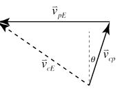
We can't use Pythagorean theorem or SOH CAH TOA because we don't have a right triangle. We need to resolve or break  $\vec{v}_{cp}$  in to its components first.
