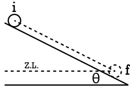
According to conservation of mechanical energy, each object starts with all gravitational potential energy and ends with translational and rotational kinetic energies.
