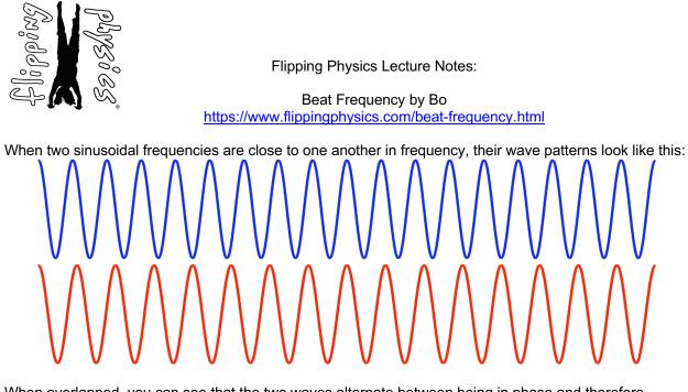
When overlapped, you can see that the two waves alternate between being in phase and therefore constructively interfering with one another to create a larger amplitude and then being out of phase and therefore destructively interfering with one another to create a smaller amplitude. When this happens, the amplitude of the two combined waves increases and decreases at the beat frequency and that is why you hear "beats".
