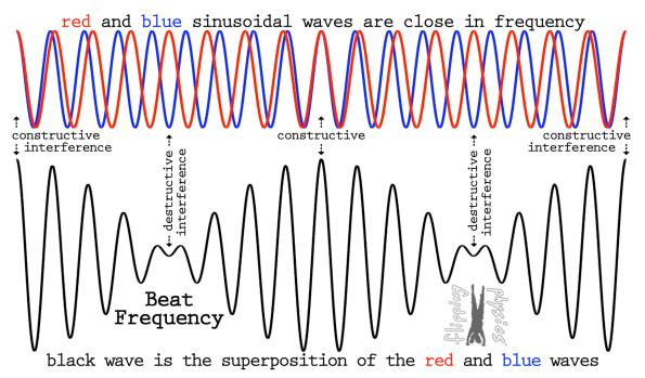
Beats can be used to tune musical instruments, like a guitar. The fourth harmonic of the low E string is the same frequency as third harmonic of the A string. If the two harmonics are played and the two frequencies are slightly off from one another, the beat frequency will be heard. You can adjust the frequency of one string until beats are no longer heard. When that occurs, the two strings are now in tune with one another.
