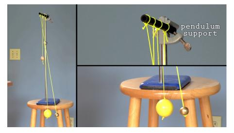
In the above picture, the oscillating brass pendulum is causing a slight motion of the pendulum support which is then causing the yellow pendulum to oscillate.
