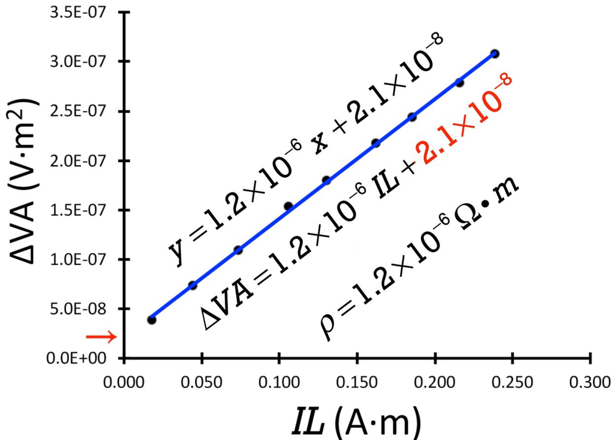
The resistivity we get from our experiment is roughly  $1.2 \times 10^{-6} \Omega \cdot m$ , which is right in the range we expect because the published value for the resistivity for nichrome at  $20^\circ C$  is in the range  $1.0 - 1.5 \times 10^{-6} \Omega \cdot m$ .<sup>1</sup>
