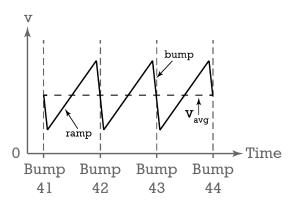
and, as the cart goes between each bump, there will be a straight line with a positive slope of a smaller magnitude. Add a dotted, horizontal line in the middle of the velocity graph and label it velocity average.
