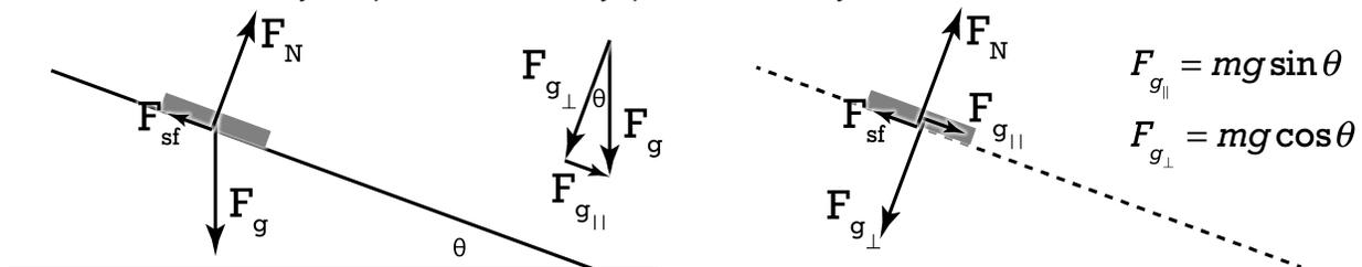
Part (b): Draw the free body diagram of the forces acting on the block as the incline angle is being increased. Break the force of gravity into its components in the parallel and perpendicular directions. Then:
