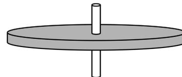
(a) At time  $t = 0$  the disk has an initial counterclockwise (positive) angular velocity  $\omega_0$ . The disk later comes to rest at time  $t = t_1$ .
