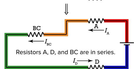
Resistor B is now removed from the circuit, and there is no connection between the wires that were attached to it. The new circuit diagram is shown.
