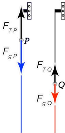
Every bit of rope below each point pulls downward on that point with a force of gravity equal to the total mass below the point times the acceleration due to gravity. A force of tension acts upward on each point. Because the rope is not accelerating, the force of tension and force of gravity are equal in magnitude at each point on the rope. Because P has more mass below it than Q, P has a larger force of gravity, and therefore a larger force of tension.
