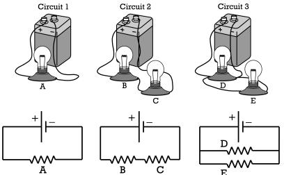
In the three circuits shown above, the batteries are all identical, and the lightbulbs are all identical. In circuit 1 a single lightbulb is connected to the battery. In circuits 2 and 3, two lightbulbs are connected to the battery in different ways, as shown. The lightbulbs are labeled A–E.
