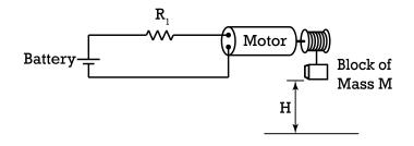
A motor is a device that when connected to a battery converts electrical energy into mechanical energy. The motor shown above is used to lift a block of mass M at constant speed from the ground to a height H above the ground in a time interval  $\Delta t$ . The motor has constant resistance and is connected in series with a resistor of resistance R<sub>1</sub> and a battery.
