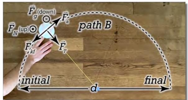
$$W_B = F_{kf} \Delta r_B \cos \theta = (\mu_k F_N) \left( \frac{C}{2} \right) \cos(180) = -\mu_k (mg) \left( \frac{\pi d}{2} \right) = -\frac{\pi}{2} \mu_k mgd \neq -\mu_k mgd = W_A$$
