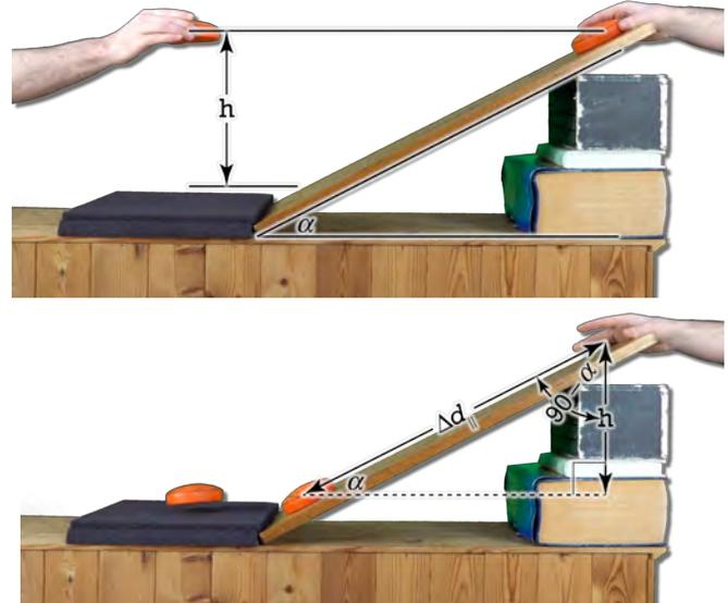
In other words, no matter the angle of the incline, the work done by the force of gravity on the object as the object goes down a distance  $h$  is the same. Because the work done by the force of gravity on an object is *independent* of the path taken by the object, the force of gravity is a *conservative force*.
