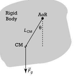
A physical pendulum is a rigid body suspended by a single point which oscillates without friction. Therefore, there is a force of gravity acting on the center of mass of the rigid body which causes a torque around the axis of rotation. The net torque around the axis of rotation is:
