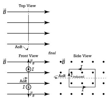
This is a very basic illustration of how an electric motor works. Current is placed through wire loops in magnetic fields which causes the loops to rotate converting electric potential energy to mechanical energy.
