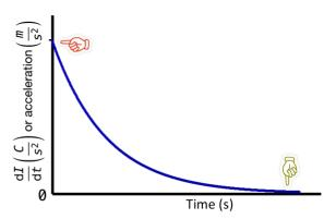
$$\Delta V_{\text{Loop}} = 0 = \varepsilon - \Delta V_R - \Delta V_L = \varepsilon - IR - L \frac{dI}{dt}$$
