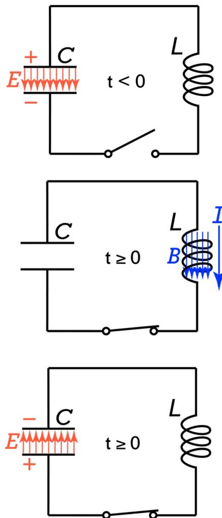
$$\Rightarrow \theta = \left(\frac{q}{C}\right) \frac{dq}{dt} + (Li) \frac{di}{dt} \quad \& \quad i = \frac{dq}{dt} \quad \& \quad \frac{di}{dt} = \frac{d^2q}{dt^2}$$
